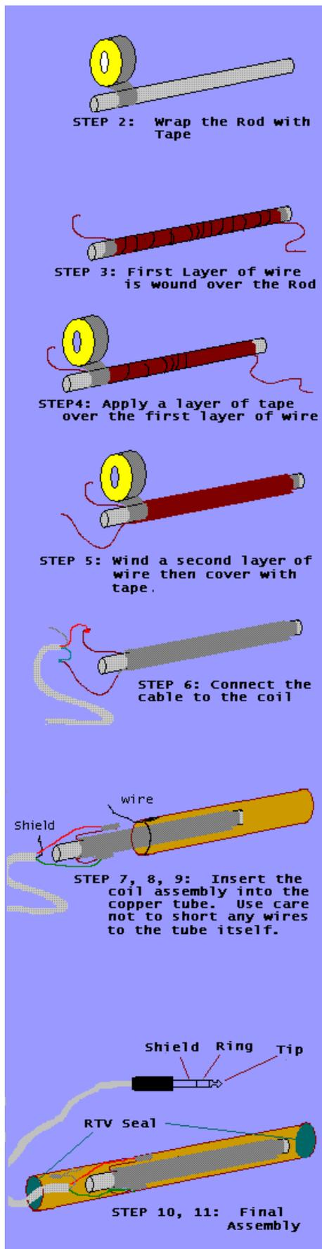
before you get it taped! Wrap a layer of tape over the entire assembly to hold the wire in place and protect it.
