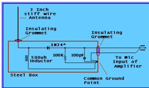
The schematic of the Raudive Diode Detector is shown to the left. Construction is quite straight forward. There are a few points to consider as you build it.
