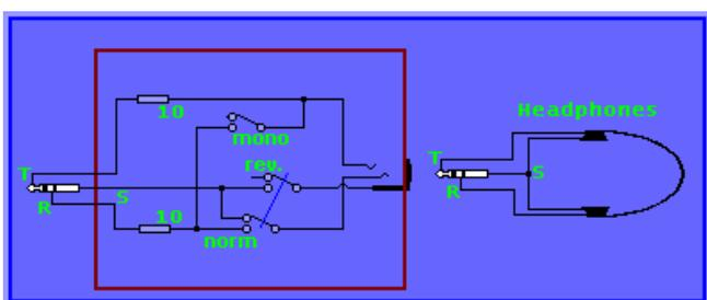
This is the schematic of the headphone adapter. Two switches are provided. The first changes the output from normal to reversed mode by placing both earpieces in series (mono) and out of phase.
